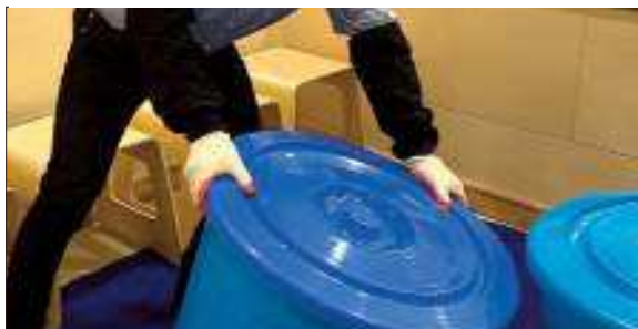
6. Close lid, roll on the side to melt the caustic potash. Be careful of small amount of gas produced.
