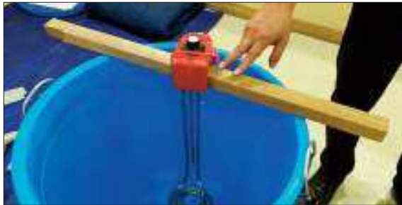
Use 3kw heater for 500 L (132 gal), 1.5kw for 100-300 L (26-79 gal).
