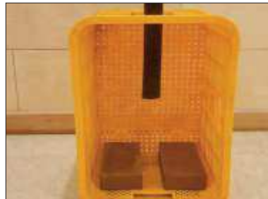
2. Place a pipe so that the opening is in the middle of the box. The pipe will be connected to an electric motor
