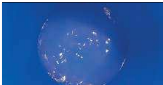
7. Heat is produced when caustic potash meets water. Make sure it has melted completely.
