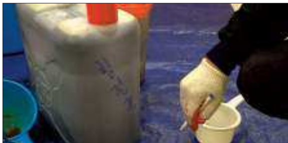
50. The storage container with sediments should be marked separately and let sit again.
