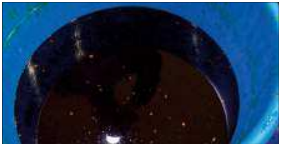
31. Sulfur has melted completely. Sulfur content is 40%. If you leave it as is, crystals will form when cold.
