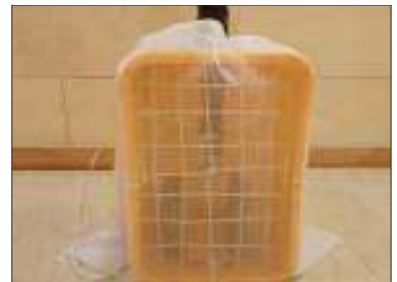
6. Tightly tie the opening of the bag. Put it in 5 t (1,320 gal) container and connect the motor.
