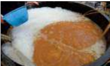
4. Use air pump so that clay will not sink down.
