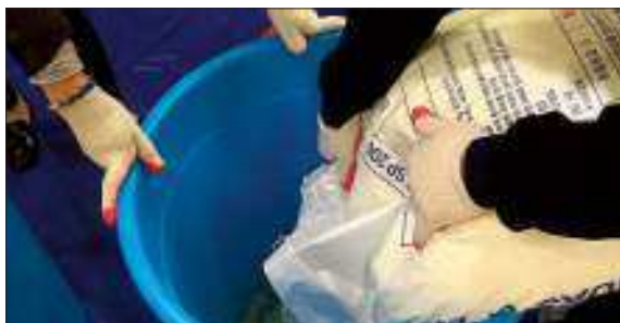
7. Add 25 kg (55.1 lb) of sulfur. Do it slowly so that dust will not rise.
