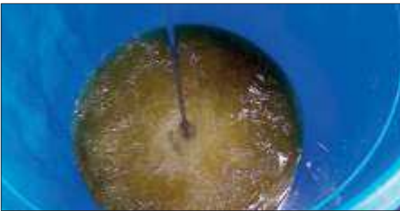
11. If you use a container that is too wide, the depth will be shallow and liquid can splash while drill-mixing
