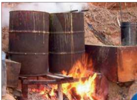
Making of lime sulfur. This needs high heat and takes a very long time. Photo: Jongsang Lee
