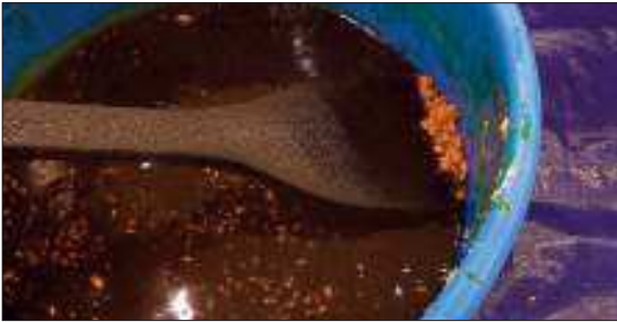
26. Keep checking the bottom to make sure no sulfur is left. Keep stirring.
