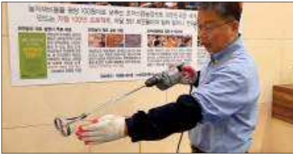
10. Prepare an electric drill. The blade must be very clean. Slower drill prolongs the mixing time.
